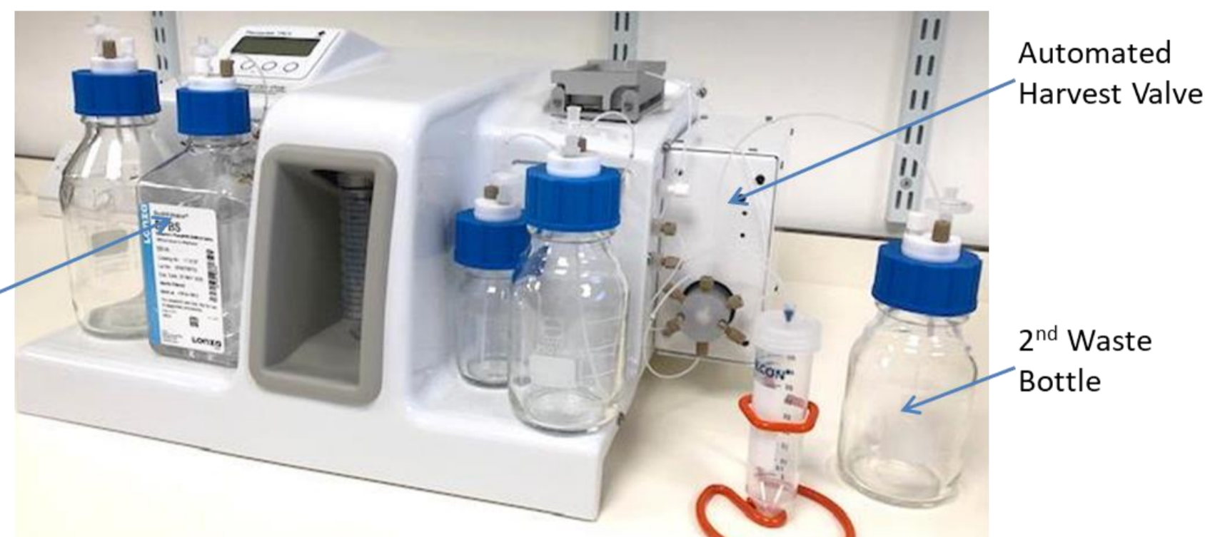
Figure 1. Modified Parsortix Instrument Parsortix instrument with a number of external modifications highlighted. Certain internal changes were also made in order to improve speed and reliability.
